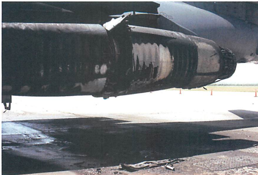
Figure 10. Left Nacelle Damage (Tab S-23)
