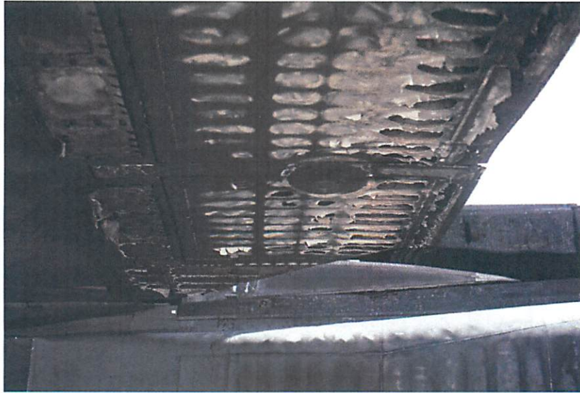
Figure 9. Left Wing Underside Damage (Tab S-14)
