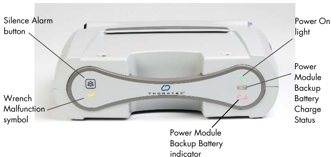
Figure 7.4 Alarm Indicators on Front of Power Module
