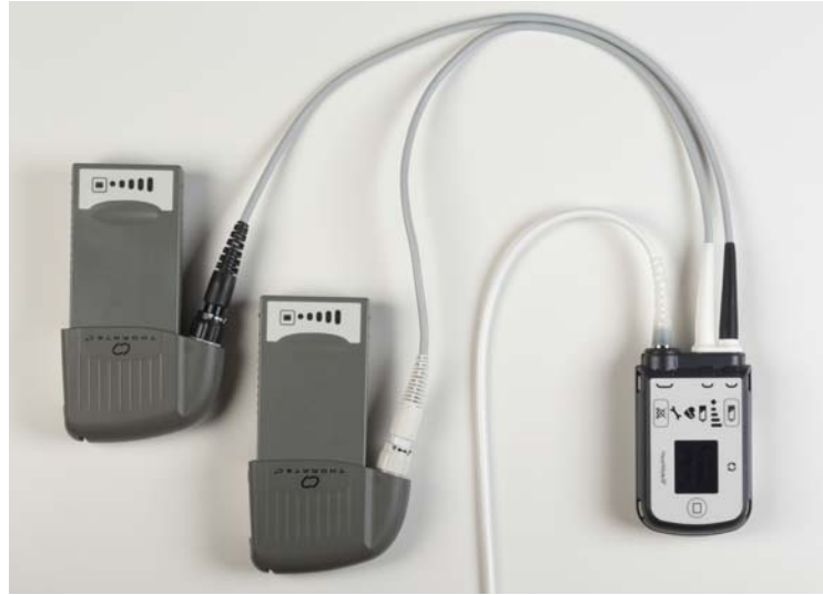
Figure 3.63 System Controller Power Cables Connected to Battery Clips
