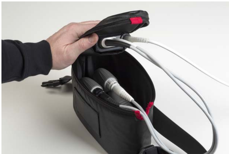
Figure 6.10 Position the Power Cables Inside the Bag
