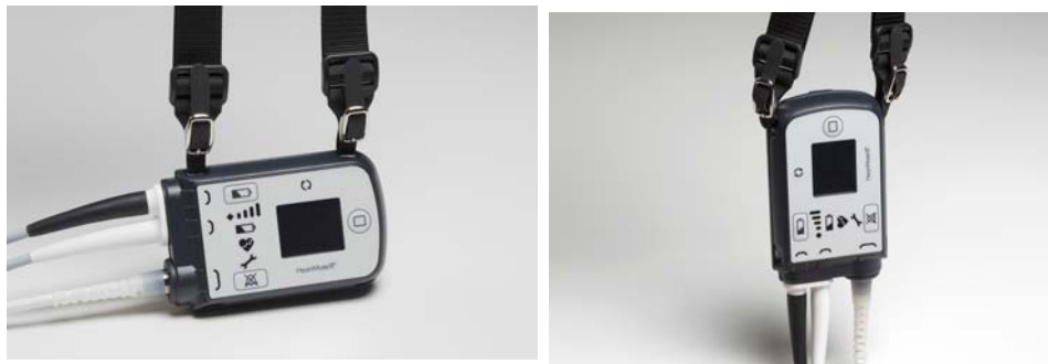
Figure 6.20 System Controller Suspended on System Controller Neck Strap Horizontally (left) and Vertically (right)
