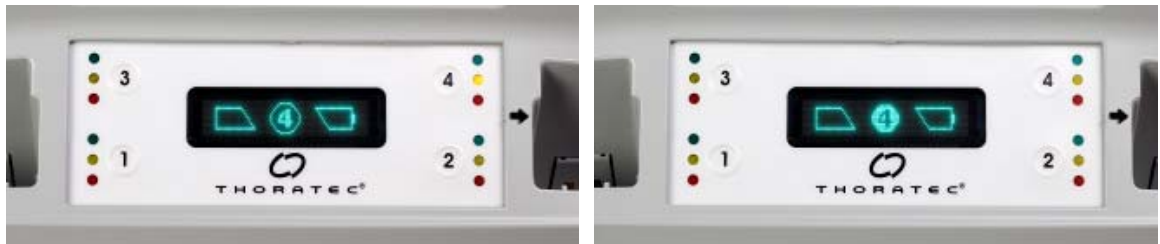
Figure 3.79 Calibration Prompt (in Graphic Mode) Indicates that the Battery in Pocket 4 Needs Calibration
