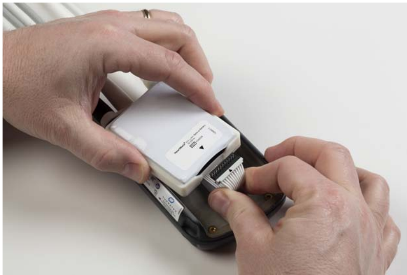
Figure 5.43 Align the Arrow on the Cable with the Arrow on the Battery
