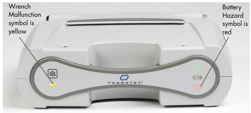
Figure 3.27 Yellow Wrench and Red Battery Hazard Symbol Indicate that the Power Module Backup Battery is Not Working — Switch to Another Power Source Immediately
