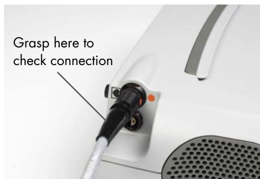
Figure 3.68 Tug on the Black Strain Relief Portion to Check the Connection
