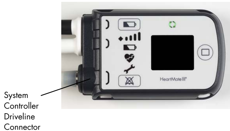
Figure 2.8 System Controller Driveline Connector on the System Controller
