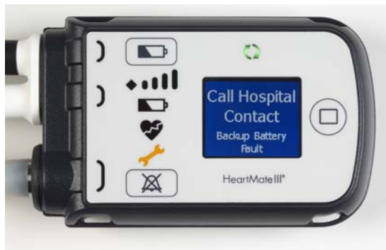
Figure 2.23 Backup Battery Fault Alarm
