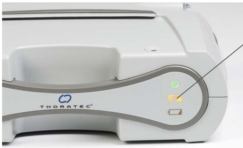
Figure 3.25 Yellow Charge Symbol Indicates that the Power Module Backup Battery is Charging
