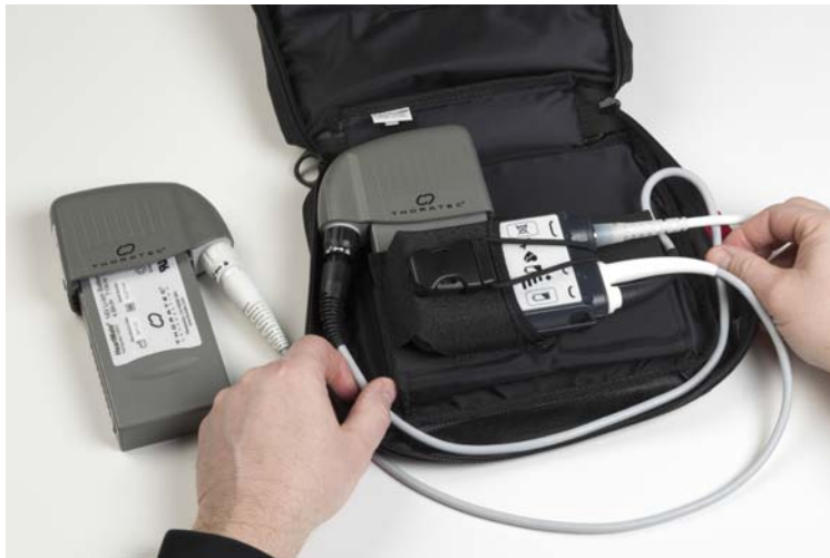
Figure 6.38 Arrange the Cables Around the Edge of the Bag
