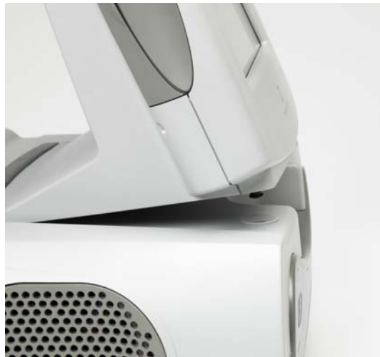
Figure 4.6 Engage the System Monitor Feet in the Grommets on the Power Module
