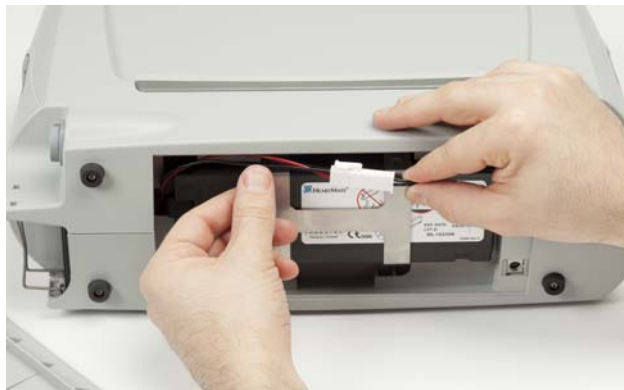
Figure 3.30 Gently Pull the Wires and Connectors Away
