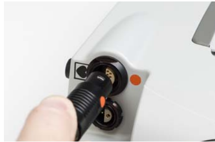
Figure 3.19 Align the Red Dot on the Connector with the Red Dot on the Power Module
