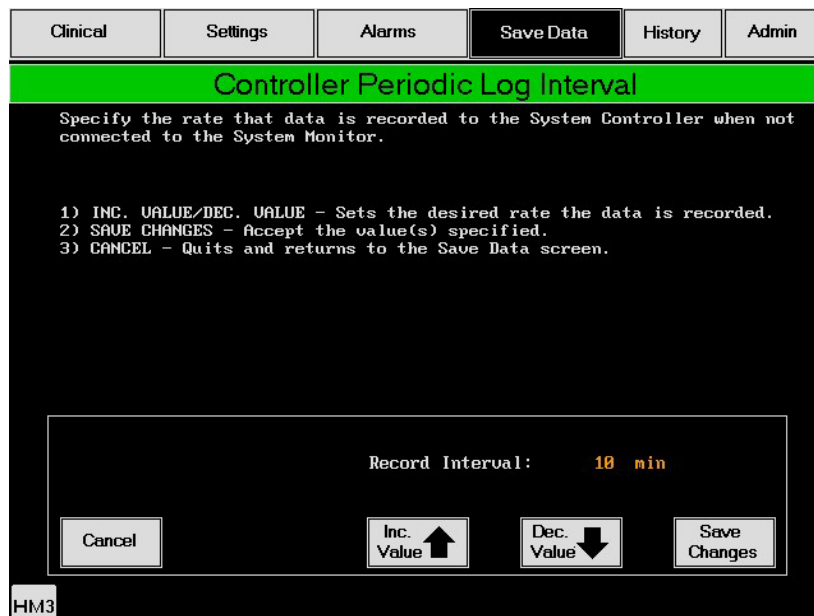
Figure 4.34 Controller Periodic Log
