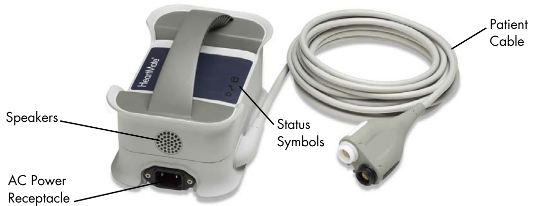
Figure 3.40 The Mobile Power Unit
