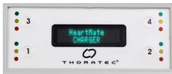
Figure 3.77 Charge Status Lights (Green, Yellow, Red) for Pockets 1 through 4
