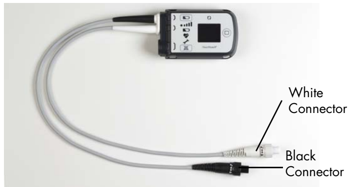
Figure 3.50 System Controller Power Cable Connectors
