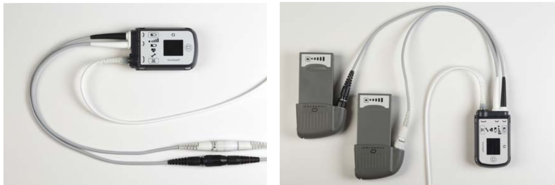
Figure 2.34 System Controller on Power Module Power (left) and Battery Power (right)
