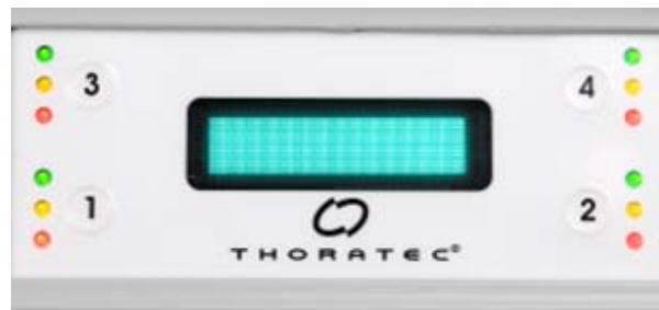
Figure 3.71 Display Panel During Battery Charger Self Test
