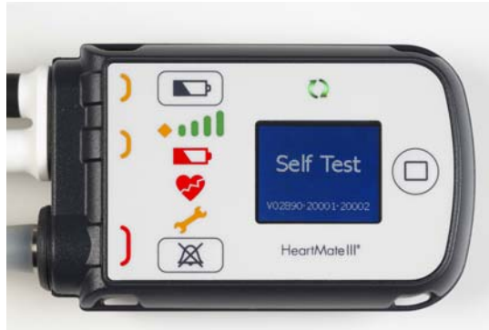
Figure 2.17 User Interface During System Controller Self Test
