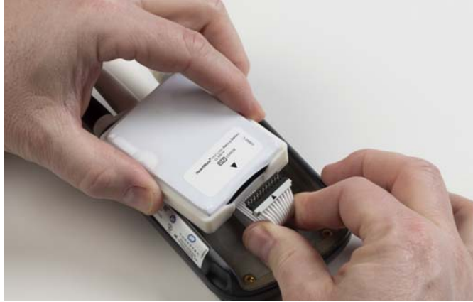
Figure 2.32 Install Backup Battery
