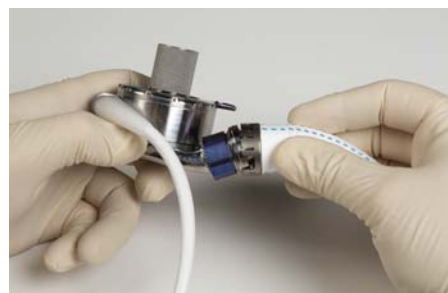
Incorrect: Not Fully Connected
