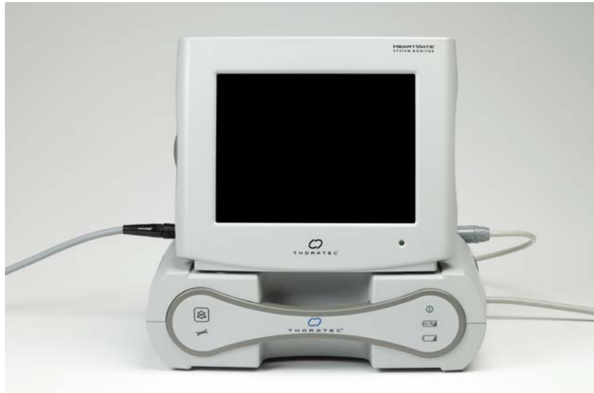
Figure 4.4 System Monitor Mounted on the Power Module
