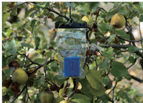
An offline AudioMoth acoustic monitoring device deployed on a fruit tree on a farm in Italy
