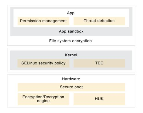
EMUI provides a secure boot mechanism in the underlying hardware chip to prevent the EMUI read-only memory (ROM) image from being tampered with. The ROM image can run on a device normally only after passing signature verification, which ensures secure boot for the boot loader, recovery, and kernel image. The Android native system provides verified boot to ensure the secure boot of the Android system and prevent tampering and malicious code implantation, thereby
