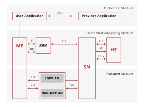
Network access security (I), Network domain security (II), User domain security (III), Application domain security (IV), SBA domain security (V)
