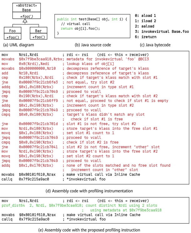
Figure 5 (a) UML diagram showing the definition of the abstract class Base and two concrete subclasses, Foo and Bar . (b) Java code of the method test , which calls the virtual method foo . (c) The Java bytecode generated for the method test . (d) Snippet of the machine code generated by HotSpot JVM — the code shown in red is responsible for profiling the virtual call. (e) Snippet of the machine code using the proposed ISA extension to profile and update the metadata of the virtual call.
