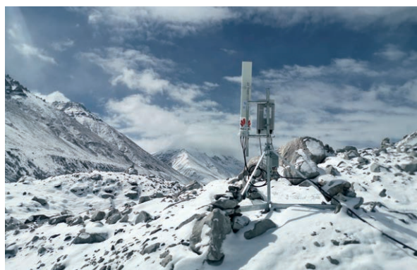
A Huawei simplified 5G site that provides gigabit access for the highest peaks of the Himalayas
