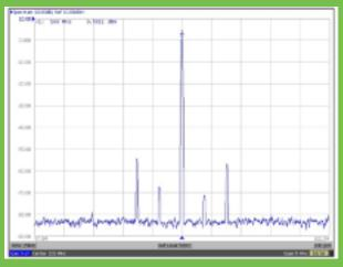
The high power of the carrier signal can result in radiated emissions and cause EMI if the circuit traces carrying the signals are not perfectly balanced and terminated. By modulating a clock with spread-spectrum, high power in a single narrow frequency band is replaced with lower power spread over a wider band. This reduces the EMI associated with the signal.
