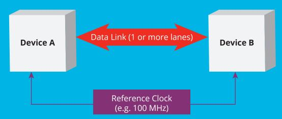
Ideally, the clock driving the Rx Latch is an exact duplicate in frequency and phase of the clock driving the Tx Latch. If this is not the case, may cause errors. The jitter of the Rx Latch clock relative to the Tx Latch clock.
