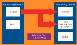
Each PCIe version specification further provides multiple possibilities for HTxPLL(s), HRxPLL(s) and  $H_{CDR}(s)$  to model various PCIe use cases. Consequently, there are many calculated  $H_{jitter}(s)$ for each PCIe version.
