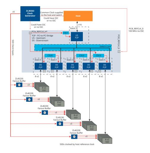
In this example, we see a ZL30263 Microchip clock generator providing the PCIe clocks for SSDs and a PCIe-to-PCIe bridge.
