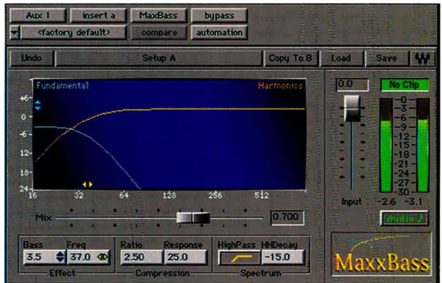
Waves' MaxxBass plug-in enhances perceived bass response by adding harmonics that create difference tones.
