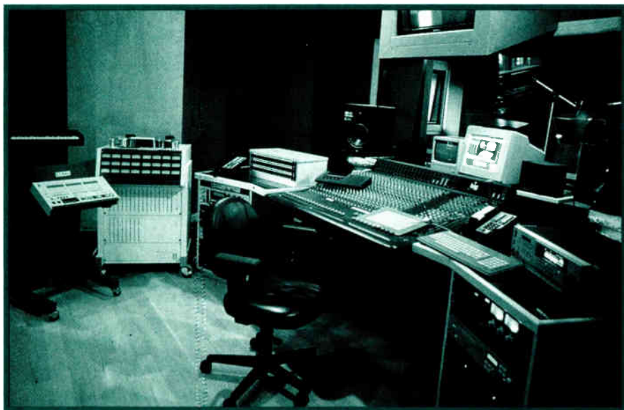
Audio 1 in: Coconut Grove features an Amek BIG by Langley console with Supertrue automation, SSL ScreenSound V.5, Otari MTR-90 24-track and Meyer HD-1 monitors.
