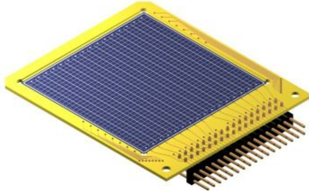
Figure 3.4: Drawing of a DSSSD with 16 strips on the front and 16 perpendicular strips on the back, which in total forms a detector with 256 separate segments. Figure from [13].
