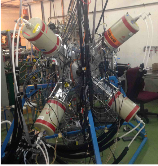
(a) The HPGe-detectors surround the rest of the setup to measure the outgoing photons, which easily penetrate through the inner parts of the setup.
