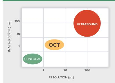
While ultrasonic inspection has become the standard in subsurface imaging, it is limited in its speed, resolution, and ability to probe small or irregular samples. Confocal imaging provides submicron resolution, but is very expensive, and limited to depths of less than 1 mm.
