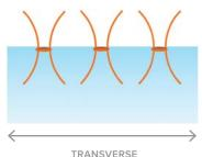
Focusing of the infrared light beam provides high transverse resolution, even at high image rates, providing a B-scan in just milliseconds.
