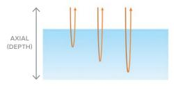
Low-coherence interferometry of infrared light is used to estimate time of flight, quantifying depth and providing micronlevel resolution.
