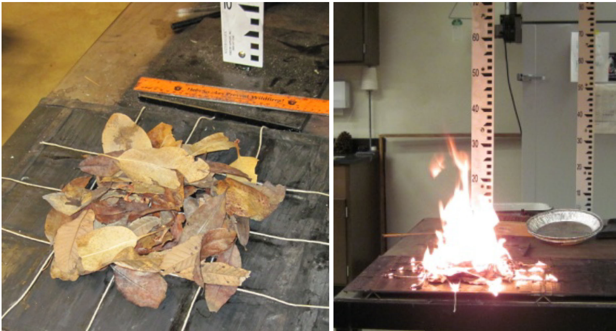
Fig. 1 Laboratory burning of litter from northwestern California forests. Litter samples were spread over a 400 cm 2 area on top of a lattice of xylene-soaked cotton string. Samples were
