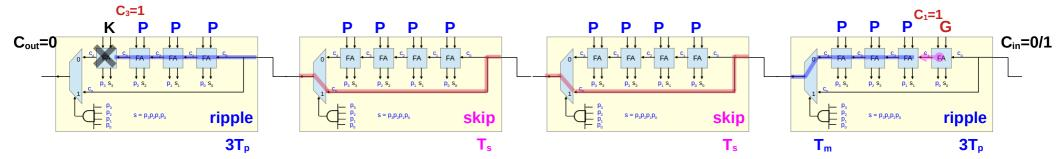
The longest delay path from  $C_1$  to  $C_{n-1}$
