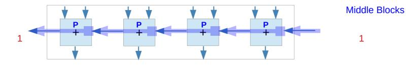
since all FA's are in the propagate mode, skip path is taken  $\rightarrow$  no ripple delay
