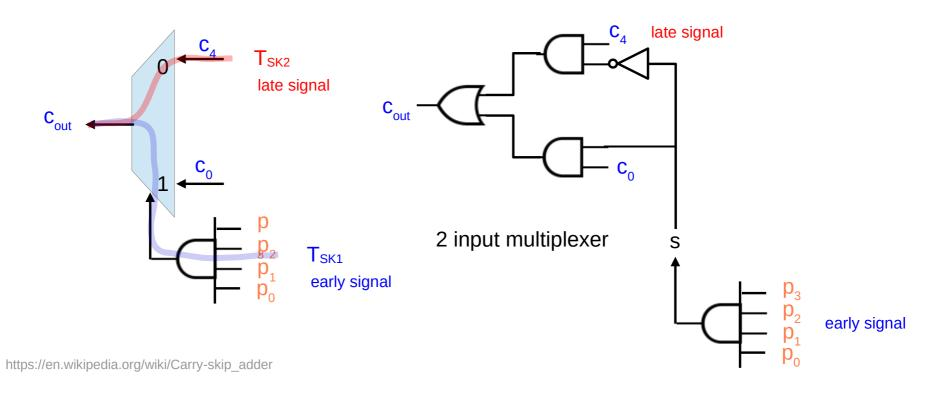
As the propagate signals are computed in parallel and are early available,
