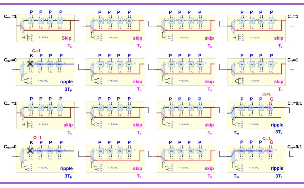
The longest delay path from C<sub>1</sub> to C<sub>n-1</sub>
