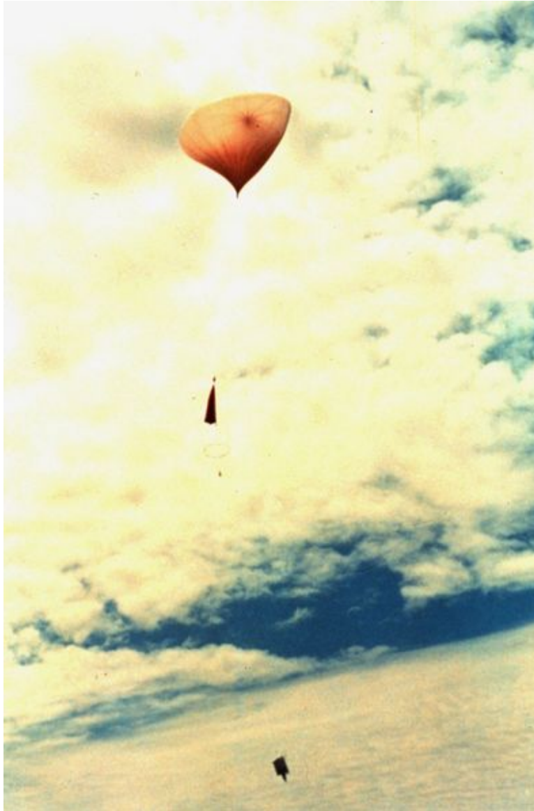
Figure 16.40: A weather balloon with a radiosonde beneath it. The radiosonde is the bottom piece and the parachute that will bring it to the ground, is above it. (39)
