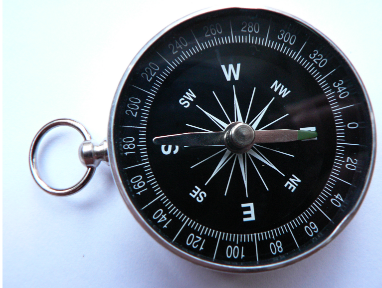
Figure 24.8: A compass; one end of the needle is pointing to the north. (11)
