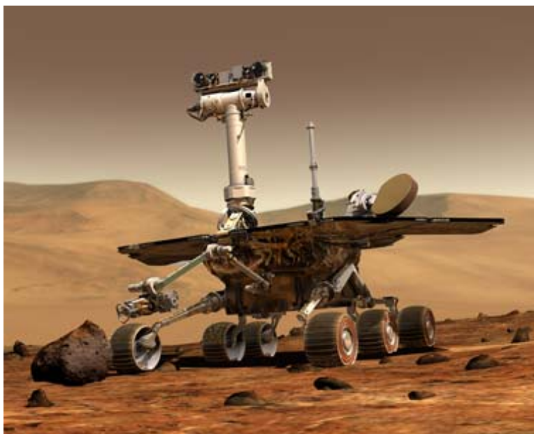
Figure 23.35: This artist's painting of one of the two Mars rovers shows the six wheels, as well as a set of instruments being extended forward by a robotic arm. (29)
