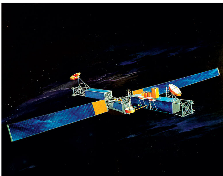
Figure 23.21: This is a Milstar communications satellite used by the U.S. military. The long, flat solar panels provide power for the satellite. Most of the other instruments you can see are antennas for sending or receiving signals. (3)
