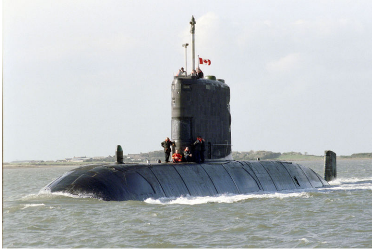
Figure 14.21: Submarines are built to withstand great pressure under the sea, up to 680 atmospheres of pressure (10,000 pounds per square inch). They still rarely dive below 400 meters. (25)
