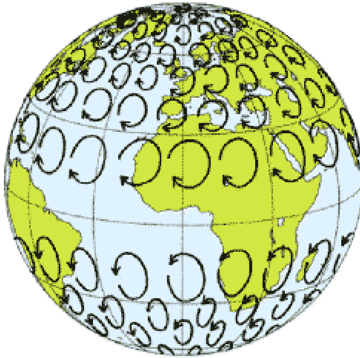
Figure 14.15: The Coriolis Effect causes winds and currents to form circular patterns. The direction that they spin depend on the hemisphere that they are in. (19)
