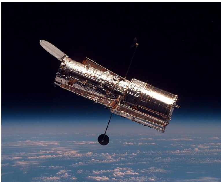
Figure 23.11: The Hubble Space Telescope orbits Earth at an altitude of 589 km (366 mi). It collects data in visible, infrared, and ultraviolet wavelengths. (12)
