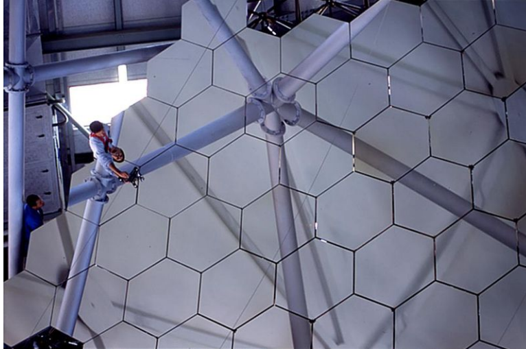
Figure 23.7: The South African Large Telescope (SALT) is one of the largest reflecting telescopes on Earth. SALT's primary mirror consists of 91 smaller hexagonal mirrors, each with sides 1 m long. (21)
