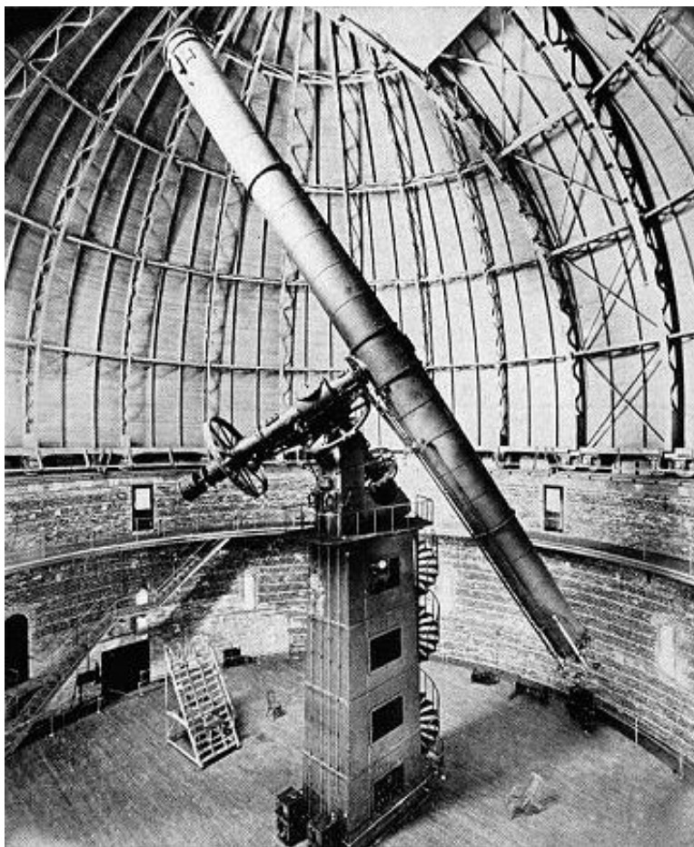
Figure 23.4: The largest refracting telescope in the world is at the University of Chicago's Yerkes Observatory in Wisconsin. This telescope was built in 1897. Its largest lens has a diameter of 102 cm. (20)
