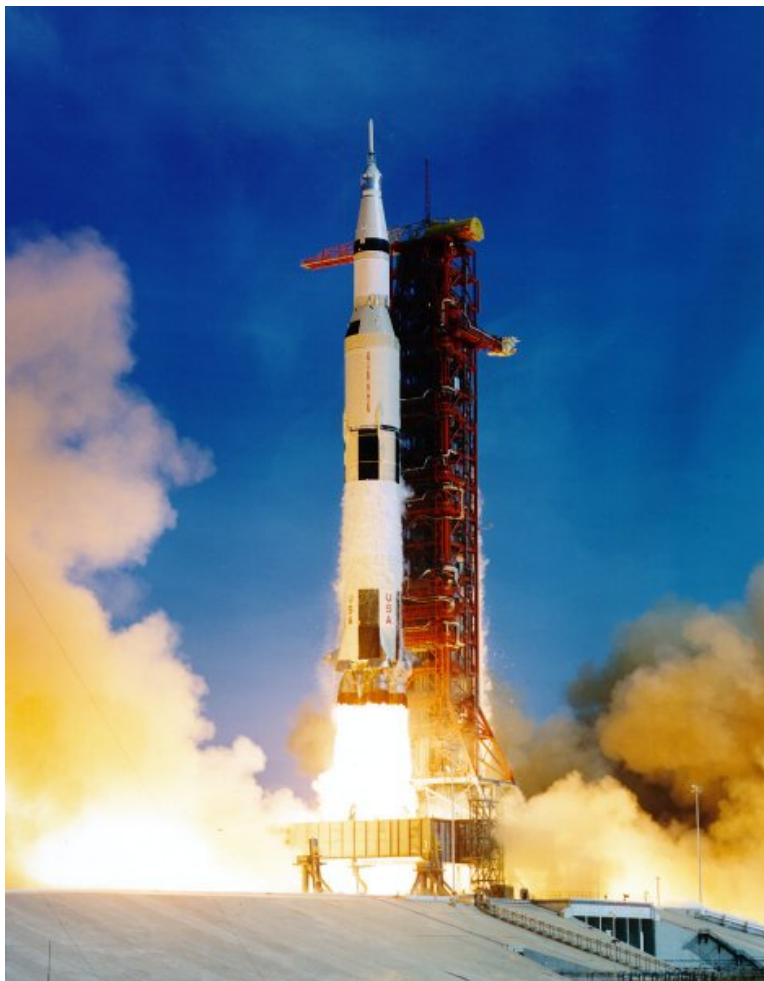
Figure 23.17: Explosions in a chamber create pressure that pushes gases out of a rocket. This in turn produces thrust that pushes the rocket forward. The rocket shown here is a Saturn V rocket, used for the Apollo 11 mission—the first to carry humans to the Moon. (4)
