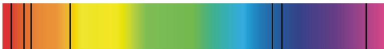
Figure 23.15: This is a simplified example of what light from a star looks like after it passes through a spectrometer. (2)
