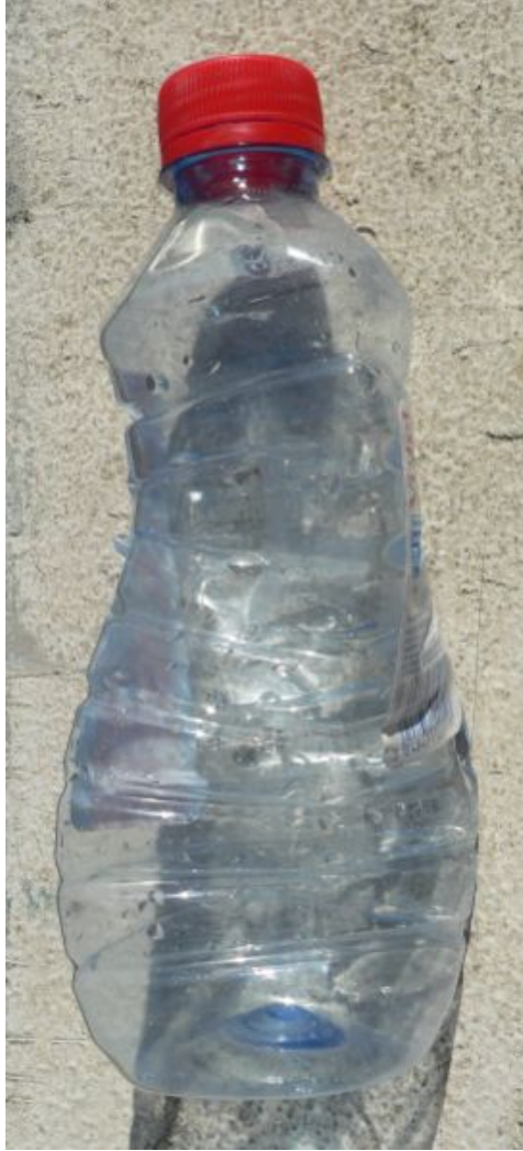
Figure 15.3: The difference in air pressure between 2,000 meters and sea level caused this bottle to collapse. The bottle was originally at higher elevation, where air pressure is lower. When it was brought down to sea level, the higher air pressure at sea level caused the bottle to collapse. (25)
