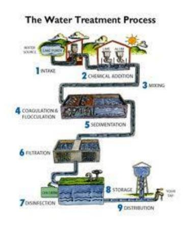
9. **Disinfection,** typically with chlorine, can be the final step before discharge of the effluent. However, some environmental authorities are concerned that chlorine residuals in the effluent can be a problem in their own right, and have moved away from this process. Disinfection is frequently built
