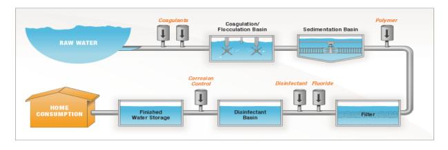
8. **Filtration** is the process of removing solids from a fluid by passing it through a porous medium. Coarse, medium, and fine porous media have been used depending on the requirement. The filter media are artificial membranes, nets, sand filter, and high technological filter systems. The choice of filters depends on the required filtering speed and the cleanness requirement. The flow required for filtration can be achieved using gravity or pressure. In
