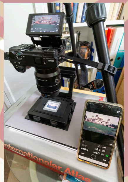
The digitization set-up: Camera with macro lens mounted on tripod. Slideholder over a flat lightbox. Smartphone as remote-control for shockproof exposure
