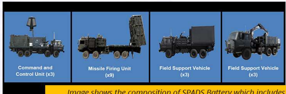
Image shows the composition of SPADS Battery which includes different kinds of vehicles with specific functions.
