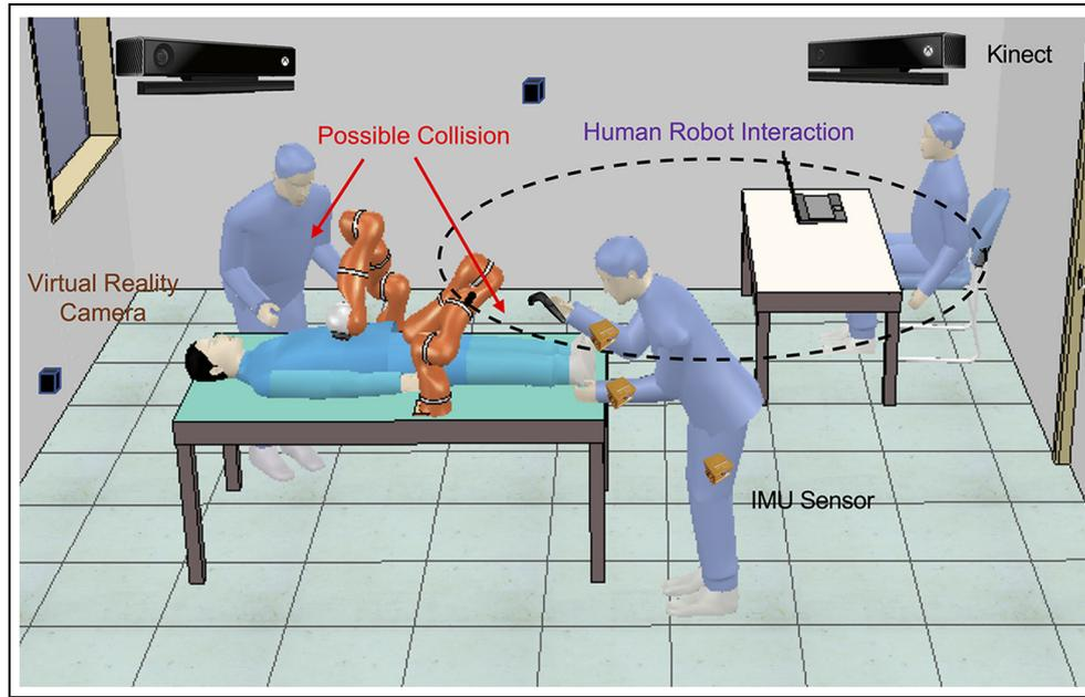
**Figure 1.** The general scenario in the operating room for human activity and hand gesture recognition using multimodal fusion-powered devices.
