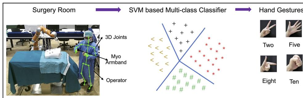
**Figure 7.** The diagram for recognizing four hand gestures using Myo armband and Kinect camera in the surgery environment.
