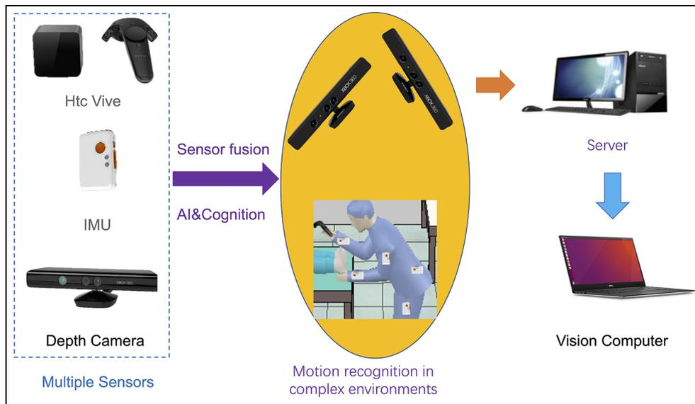
Figure 5. The hardware system structure for data collection and processing.
