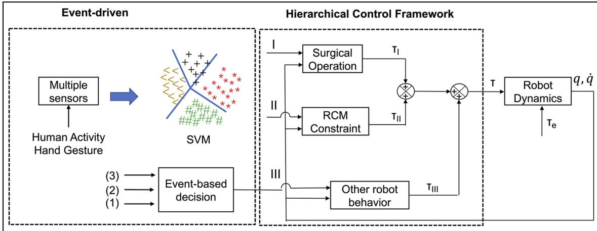
Figure 4. The event-driven scheme based on control model and SVM classifier.
