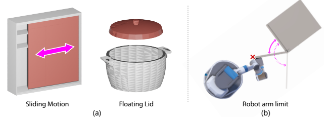
Fig. 13. Failure cases of our method. (a) Two kinds of objects that our method fails to reconstruct due to the unsupported movement of the gripper or freeform motion of the non-articulated part; (b) A top-down view of a robot opening a door where the opening angle fails to reach its maximum range due to the arm limit.
