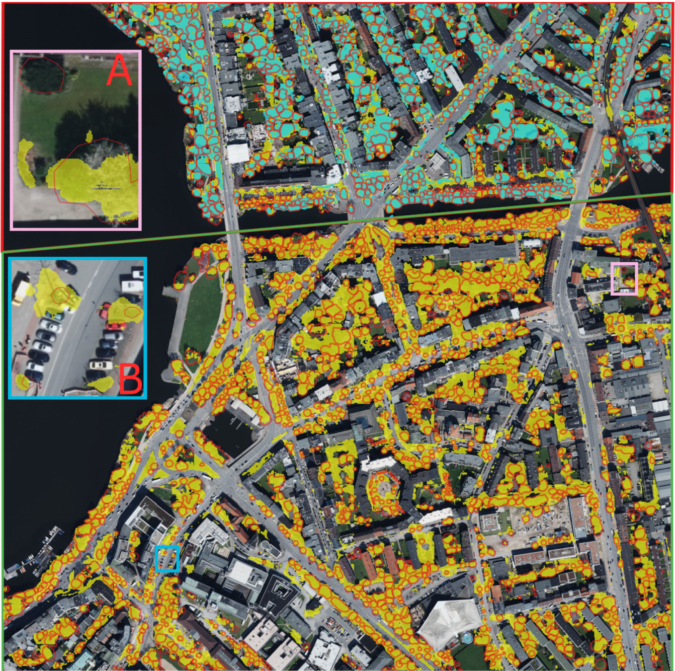
Figure 5: Results on the fully delineated dataset. Red polygons are the manually annotated ground truth. Validation data is shown within the red bounds, which is used for the model selection. As discussed in Section 5, the Mask model is the final model chosen for prediction, which shows as the yellow mask on top of the satellite image. The segmentation mask in green are from the model MaskObjThresh . The area bounded by the green lines shows the test set. Within the test area, we only apply Mask . In cutout A the model predicts one of the trees correctly and interestingly does not predict the shadow of said tree. This tree is also of bright color since it is in bloom making it a hard example. However, the second tree in top left corner was not found, possibly because the coloration is close to the one of shadows. After manual rechecking of the predicted tree in left lower corner, we found that there is a tree not annotated originally (e.g., a false negative label). Cutout B is interesting because it contains trees without leaves. The model annotated these trees effectively and even finds another tree that was missed by the annotators (bottom right). This also demonstrates how difficult it is to define clear boundaries for these trees.
