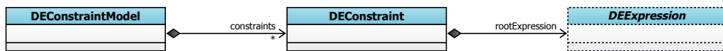
Figure 7.10.: Metamodel for the version-aware constraint language formulated in EMF Ecore. The metaclass DEExpression is defined in Figure 7.9.
