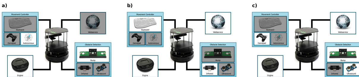
Figure 1.3.: Example of three different valid configurations of the TurtleBot driver software.
