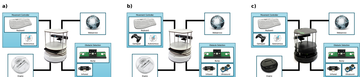
Figure 1.8.: Change of the functional components of the TurtleBot driver software over the course of approximately 1.5 years of development: a) after first development stage, b) after second development stage and c) after third development stage.
