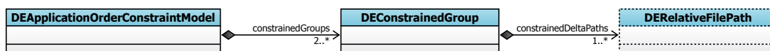
Figure 7.13.: Metamodel for application-order constraints formulated in EMF Ecore. The meta-class DERelativeFilePath is defined in Figure 7.2.
