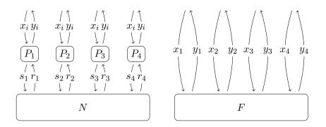
Figure 1: A multiparty protocol  $P_1, \ldots, P_4$  with communication network N (left) implementing a functionality F (right).
