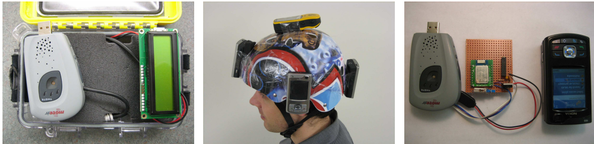
(a) Initial prototype of a BAN local display. (b) Ground truth video/sound/photo helmet with four N80s and GPS receiver. Each N80 can act as a mobile SAP. (c) BikeNet mobile SAP implementation. The Nokia N80 Bluetooth radio associates with a custom-built Bluetooth/802.15.4 gateway.
