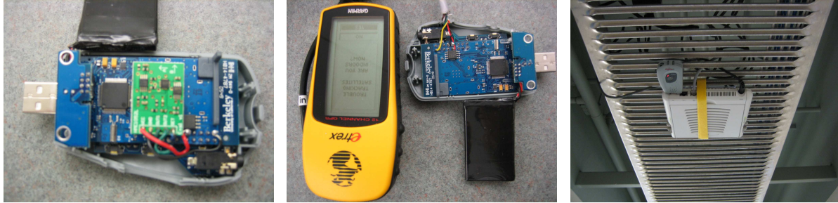
(a) Modifications to attach a two-axis magnetometer to a Tmote Invent via the ADC. (b) Modifications to attach an external GPS unit to a Tmote Invent via the UART0 port. (c) BikeNet static SAP implementation.
