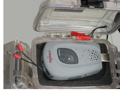
Figure 5: Waterproof OtterBox. wires connected to the user button of the Invent from the reed relay mounted next to the pedal go through a hole drilled in the waterproof Otter Box. The hole is then filled with silicone sealant. Wires have crimped connectors for easy disconnect and removal for mote recharging.
