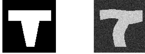
Figure 1. Template T-shape image on the left and noisy T-shape Reference image on the right.
