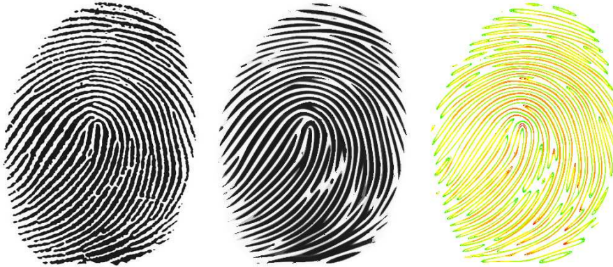
FIG. 6.17. Original fingerprint, Level Lines Affine Shortening and its Curvature map.
