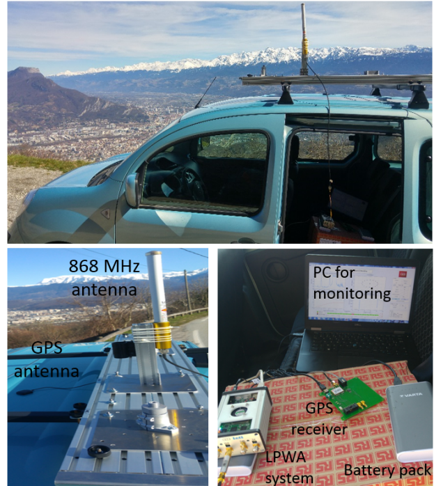
Fig. 6. Set-up of the receiver hardware and associated PC within the Field test Vehicle.
