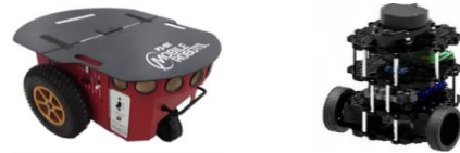
(a) Pioneer 3DX mobile robot (b) TurtleBot3 Burger Fig. 13. Experimental Setup at ACM Lab, Dalhousie University
