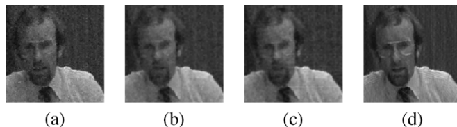
Fig. 6. Output of the filtered Trevor White third frame 256 \times 256 corrupted by mixed impulsive ( p = 5\% ) and Gaussian additive noise ( \sigma = 20 ), (a) output of the 3 \times 3 \times 3 AWA filter, (b) output of the 3 \times 3 \times 3 median filter, (c) output of the 3 \times 3 \times 3 NLMS L -filter with ( \mu_0 = 0.8 ), and (d) output of the 3 \times 3 \times 3 NLMK L -filter with ( \mu_0 = 10^{-4} ).
