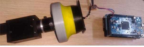
Fig. 6. Measurement setup: a camera with the attached LED source, and the signal generator implemented on an Arduino Due microcontroller unit.
