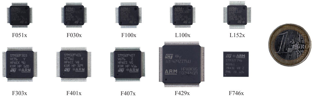
Fig. 7. Microcontrollers used in the cross-platform comparison, size-compared to a €1 coin.
