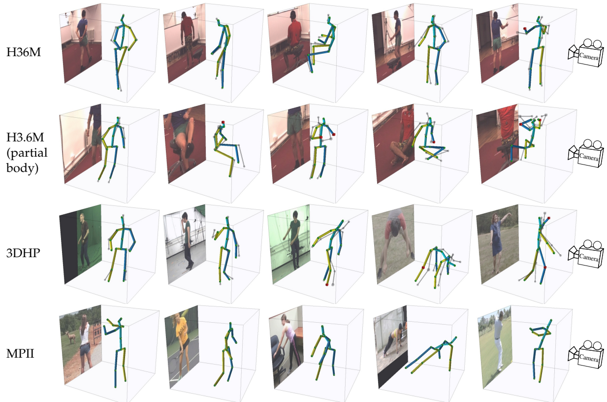
Fig. 7. Qualitative results on various datasets. Predictions are shown in color, ground truth in gray (except for MPII, where it is unavailable). Green spheres mark predictions within 150 mm of the ground truth, red cubes beyond that threshold. Note that our method performs well on truncated (partial body) images as well (second row).
