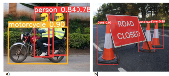
Fig. 2. Motorcycles, persons and cones detection with Yolov5; a) original image from [4] b) original image from [5]
