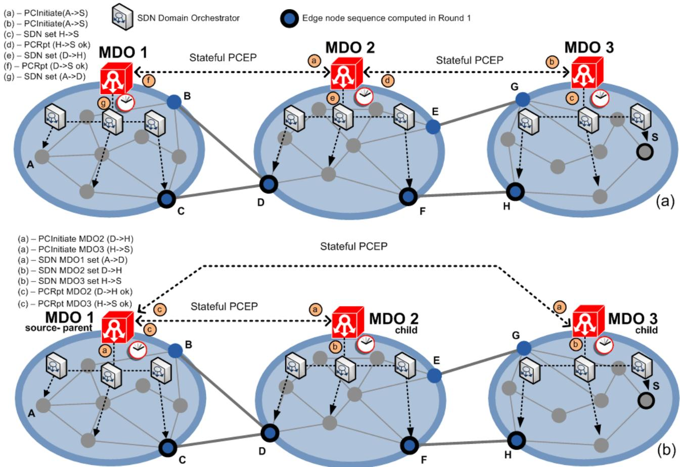
Fig. 1. Proposed architecture: peer (a) and source-hierarchical (b) procedures, for establishing inter-provider connectivity.
