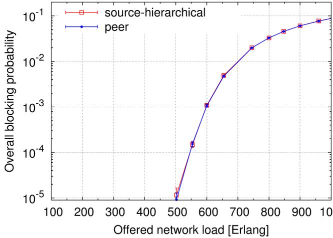
Fig. 3. Simulation results: connection blocking probability vs. offered network load.
