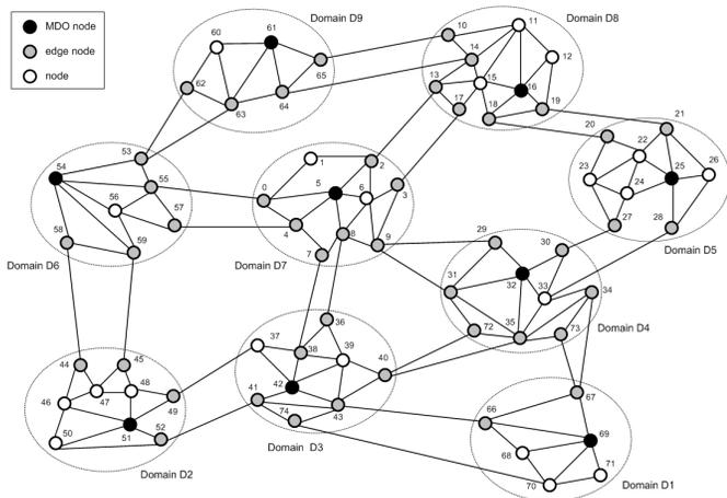
Fig. 2. Multi-provider EON test network topology.
