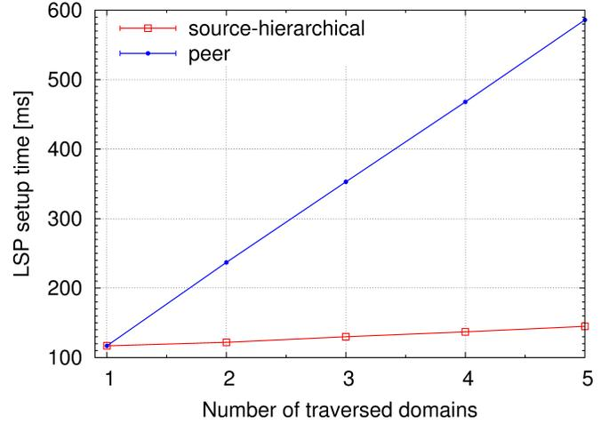
Fig. 5. Simulation results: connection establishment time vs. number of traversed providers.
