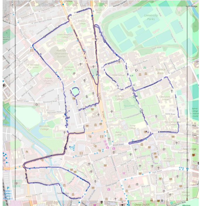
Figure 3. Samples of vehicle position are overlaid on a digital map using GPS coordinates. Although the dataset is a complete loop, we observe many gaps along the route.
