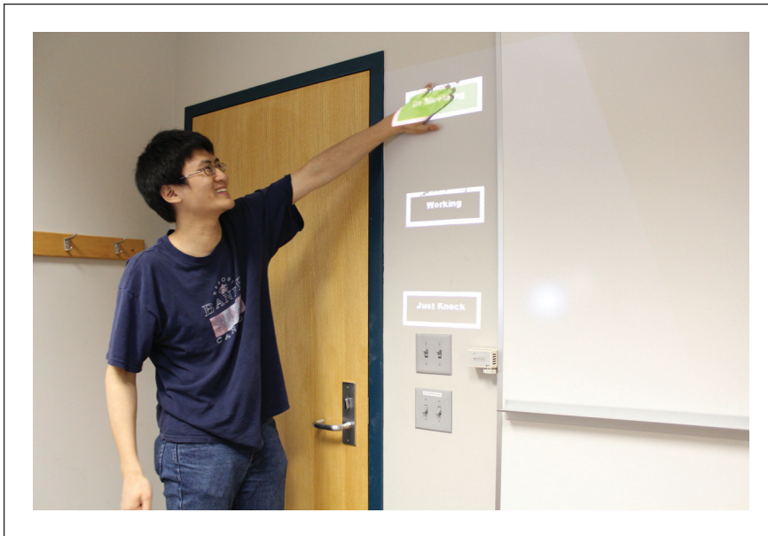
Figure 3. WorldKit combines a projector with a Microsoft Kinect to let developers put touchable user interfaces on any surface. (Source: Chris Harrison and Robert Xiao; used with permission.)
