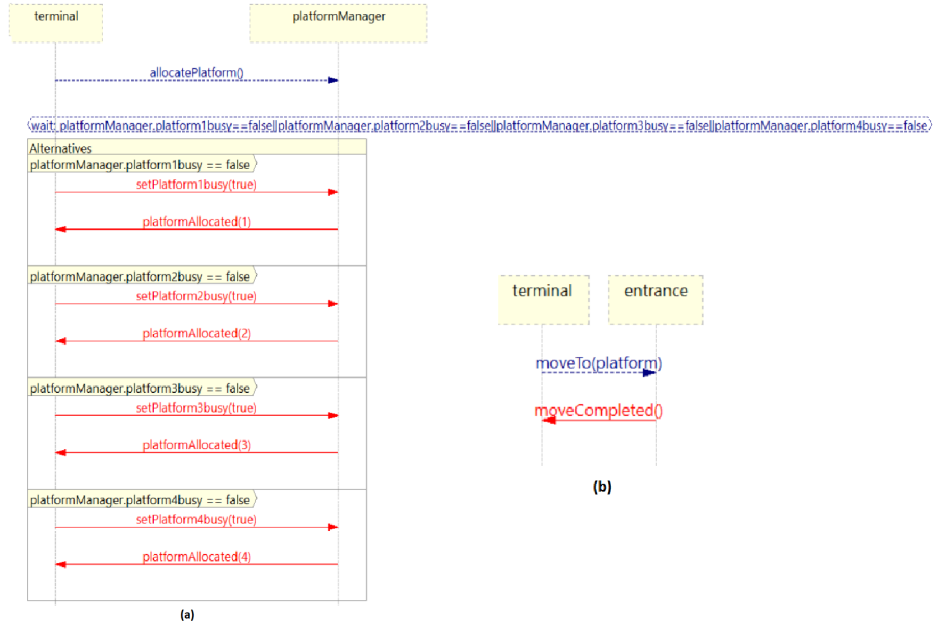
Fig. 11. (a) Platform Allocation: : the platform manager waits for some platform to become available, allocates the first available platform and marks it as busy (b) A simple LSC handling the handshake between the terminal and the entrance.
