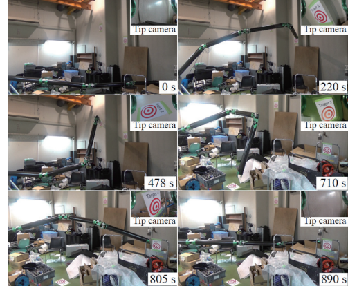
Fig. 14. End-point control experiment to capture the target markers.
