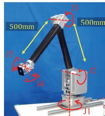
Fig. 3. 5-DoF light duty arm [11]: the three distal joints (J3, J4, and J5) are driven by wires, and their actuators are installed in the square-shaped boxes.
