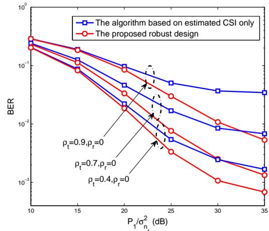
Fig. 5. BERs of proposed robust design with M-Schur-convex objective functions and the algorithm based on estimated CSI only with different  $\rho_t$ , when  $\rho_r = 0$ ,  $\sigma_e^2 = 0.002$  and  $P_2/\sigma_{n_2}^2 = 30$ dB.
