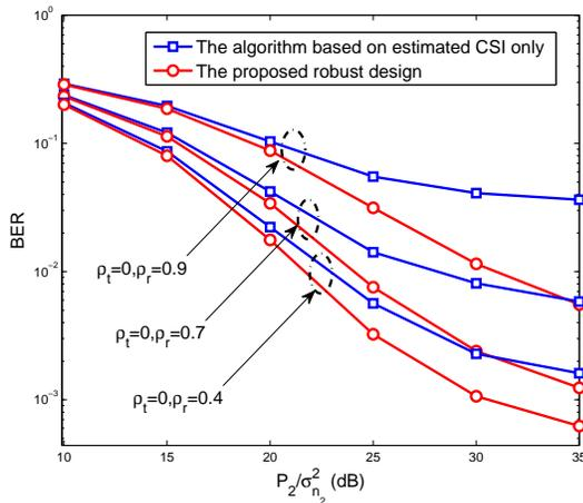
Fig. 4. BERs of proposed robust design with M-Schur-convex objective functions and the algorithm based on estimated CSI only with different  $\rho_r$ , when  $\rho_t = 0$ ,  $\sigma_e^2 = 0.002$  and  $P_1/\sigma_{n_1}^2 = 30$ dB.
