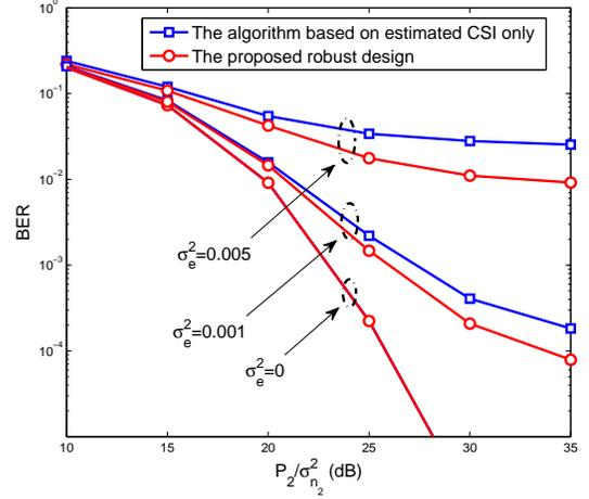
Fig. 3. BERs of proposed robust design with M-Schur-convex objective functions and the algorithm based on estimated CSI only when  $\rho_t = 0.5$ ,  $\rho_r = 0$ , and  $P_1/\sigma_{n_1}^2 = 30\text{dB}$ .
