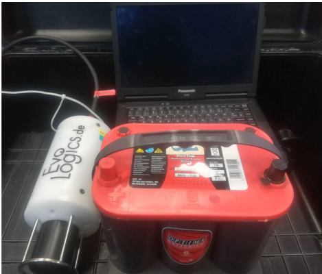
Fig. 5. Picture of the apparatus used in the experiment. Each node was equipped with batteries, a laptop and an acoustic modem.
