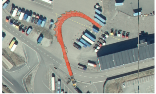
Fig. 7: GUI for creating reference paths for a parking scenario where the driver starts in the lower part of the figure and wants to park the trailer in between the other two trailers next to the end position. The yellow dots connected by the yellow lines represents the reference path. For this manoeuvre the user has only used two control points to create the simulated manoeuvre shown.
