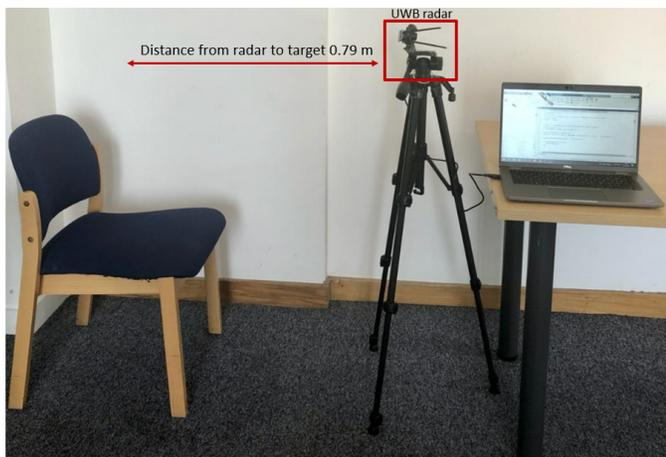
Fig. 2: Experimental setup of the proposed Head movement recognition system.
