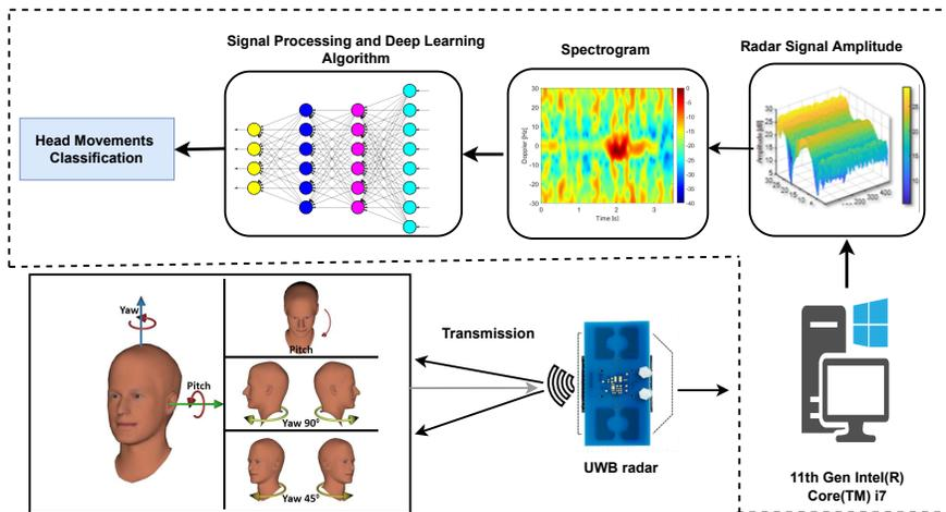
Fig. 1: Block diagram of the proposed architecture showcasing the UWB radar-based system, data gathering, and DL classification model for Head Movements.
