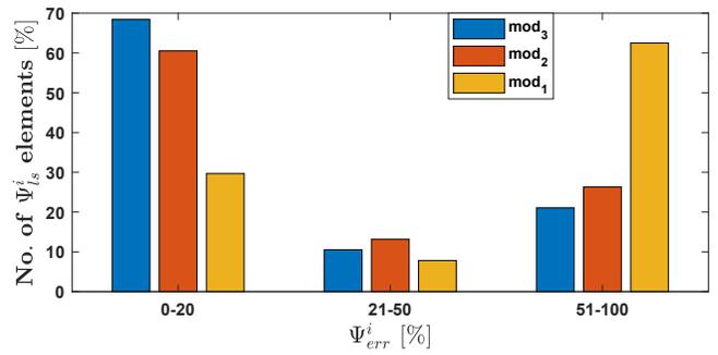
Fig. 5. The  $\Psi_{err}^i$  is categorized into three categories (0-20%, 21-50%, and 51-100%) and the percentage of  $\Psi_{ls}^i$  elements falling under each category is compared across three models:  $mod_1$ ,  $mod_2$ , and  $mod_3$ .
