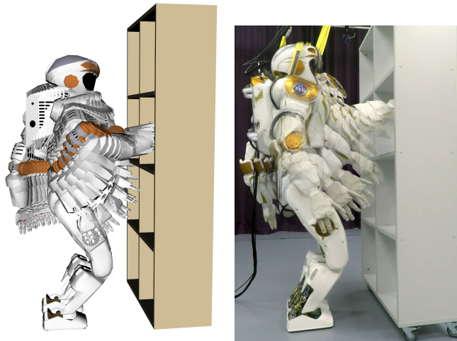
Fig. 1: Continuous time collision avoidance during whole-body manipulation execution on the 38-DoF NASA Valkyrie humanoid platform: Discrete metrics will consider a coarsely discretized trajectory to be valid while a transition between two states can be in collision with the environment. Continuous collision avoidance for discrete trajectories successfully avoids the obstacle and guarantees continuous-time collision safety.
