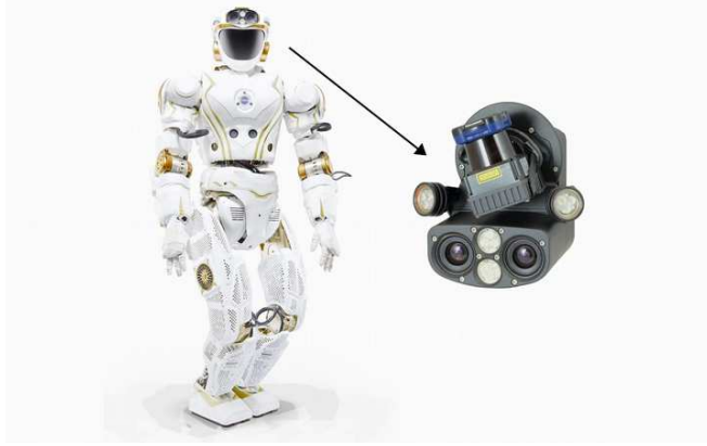
Fig. 2: The NASA Valkyrie is an 1.8m tall electrically actuated humanoid robot. Within its head is a Carnegie Robotics Multisense SL which combines a rotating LIDAR sensor and a stereo camera. The sensor is inverted on the robot. (photo credits: NASA and CRL)
