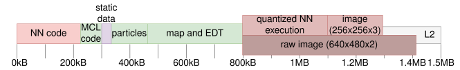
Fig. 6: The 1.5MB L2 memory on GAP9 is used for code and data.
