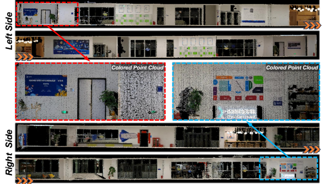
Fig. 1. The RGB-Colored point cloud reconstructed by our mobile mapping system. A fly-through rendered image from the point cloud's left and right sides.
