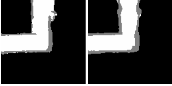
Fig. 4: Predicted occupancy map generated without class balancing weight (Left) and with class balancing weight (Right) where white represents unoccupied space, grey is occupied and black is unknown. The class balancing weight produces stronger edges for obstacles in the predicted occupancy map.
