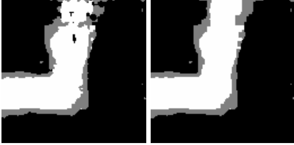
Fig. 5: (Left) Generated occupancy map with noise artifacts. (Right) Predicted occupancy map after morphological close operation (white is unoccupied space, grey is occupied and black is unknown).
