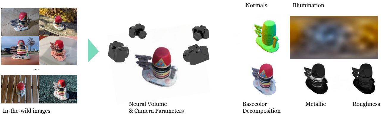
Figure 1. Object reconstruction using SHINOBI. SHINOBI decomposes challenging in-the-wild image collections into shape, material and illumination using a neural field representation while also optimizing camera parameters. Visit the project page at Project page: https://shinobi.aengelhardt.com
